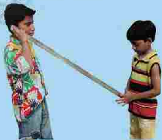
Fig. 10.12 : Sound travelling through a metre scale
