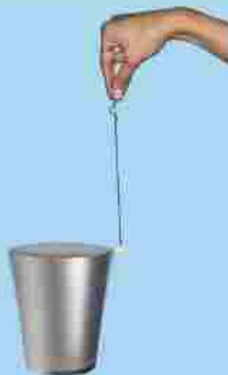
Fig. 10.17 : Thermocol ball touching the vibrating glass tumbler
