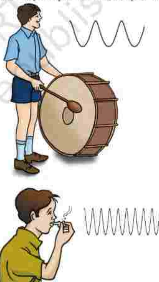
Fig. 10.18 : Frequency determines the pitch of a sound
